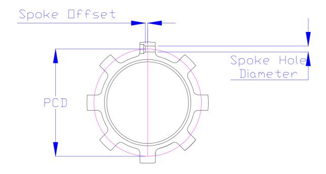
Figure showing Spoke Diameter, Offset and PCD
